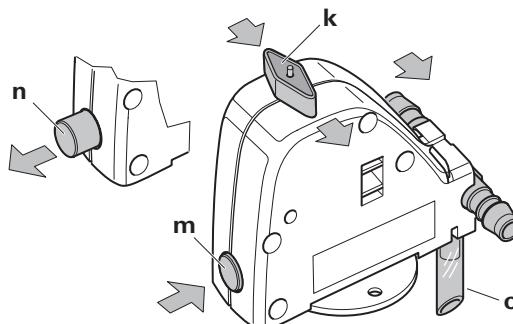
k = rotary switch position "Operation"
