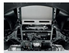
Front axle. The front axle can also be equipped with a 100% differential lock upon demand. To ensure optimal brake force distribution, it has an additional hydraulic dual-circuit brake with vacuum booster.
