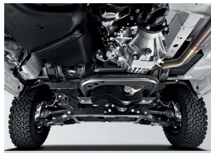
Transfer case. A separate 3-speed transfer case has been implemented for the permanent four-wheel drive in addition to the 6-speed manual gearbox. This transfer case distributes the engine power 50:50 between the front and rear axle. The integrated gear reduction level of 1:2.5 as well as the 100% differential lock can be actuated electrically from the cab when needed. The transfer case is mounted behind the front axle.
