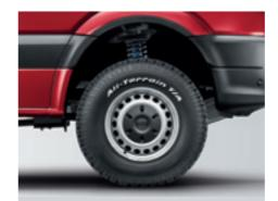
Front axle suspension. In contrast to the Crafter standard model with leaf springs, the Crafter 4MOTION has independent suspension with coil springs. These are compression springs with integrated shock absorbers and an enhanced stabiliser.
