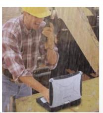
The CF-18 offers outstanding practical performance under real-world conditions. Rubber packing that is 1.5 times as thick as that of conventional models complies with IP54 water-and dust-proofing standards to assure reliable operation, even in rainy or dusty field environments.
